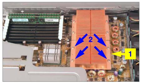
Figure 10: Installing the heat sink
